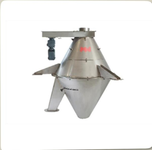
The Rotary Tube Divider (RTD) is designed for representative mass reduction of bulk material. The RTD can be used for mass reduction of virtually any type of dry materials.
